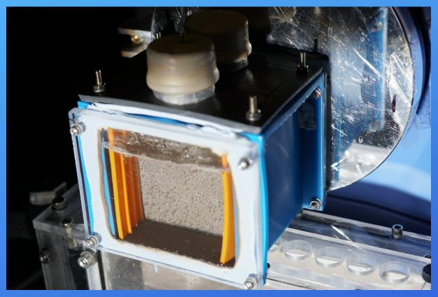
Researchers have developed a standalone device that converts sunlight, carbon dioxide and water into a carbon-neutral fuel, without requiring any additional components or electricity.
