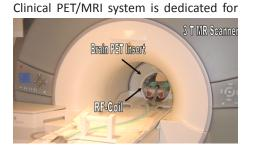
brain applications and features 3-T MRI system with dedicated head coil and PET head insert with 18-cm axial field of view.
