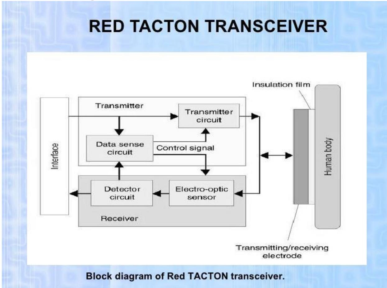
Like digital signals, the signals will depend on the fluctuations in the electric field that is induced in the body. As the electric field is mild in nature, highly sensitive sensing technology is used in the receiver part.
