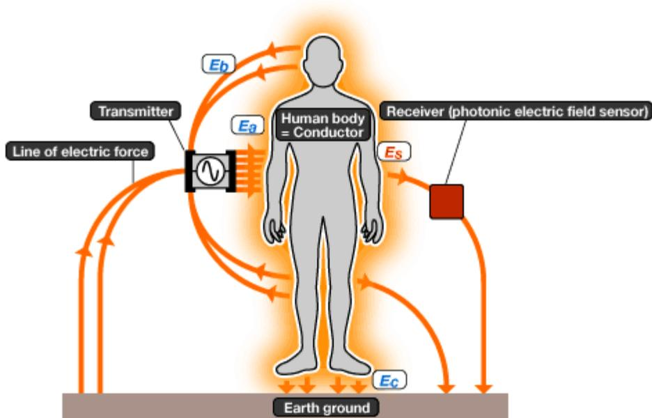
Other than the electric field that transmits the data, there will also be very small and unstable electric fields on the surface of the body. This will be natural in nature and will be automatically sent back to earth.
